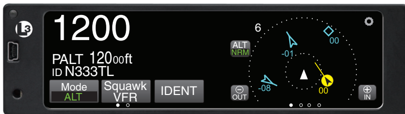
Figure 1-1: Example of Panel Mount Lynx NGT-9000
